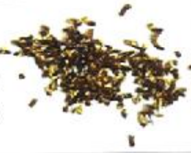
Fig. 22: Al-bronze chips of conventional and improved material at same machining conditions
