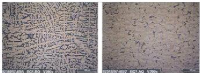
Fig. 7: Microstructure of permanent mould cast (left) and spray-formed (right) CuSn16
