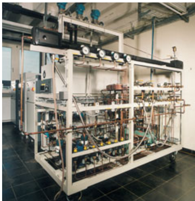
Test plant for tubes and heat exchangers
