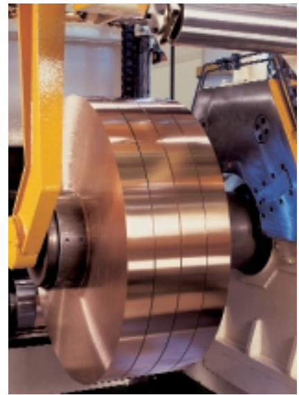
Copper strip is a high-quality pre-material for the production of coaxial cables.
