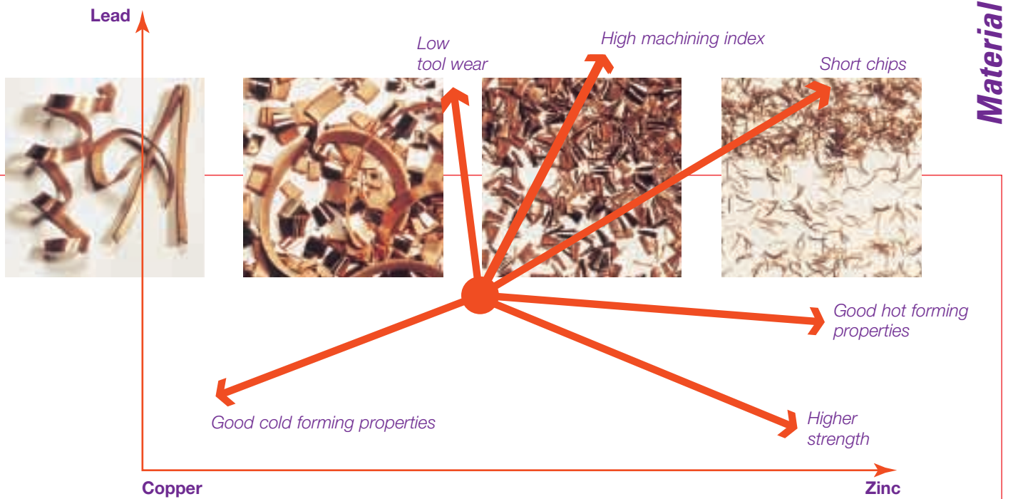
Trends of various brass properties depending on the zinc and lead content
